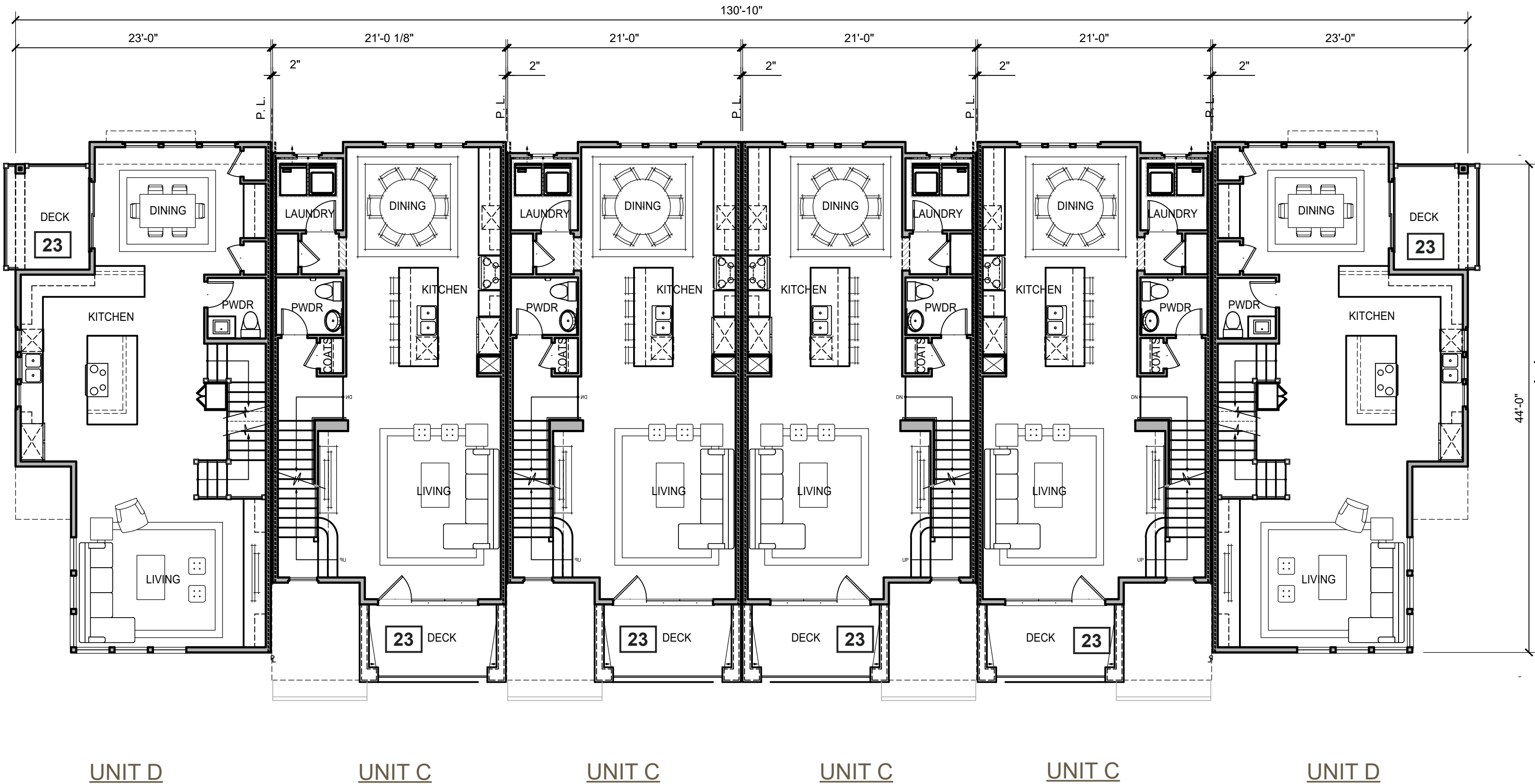
6-PLEX_2: SECOND FLOOR PLAN
