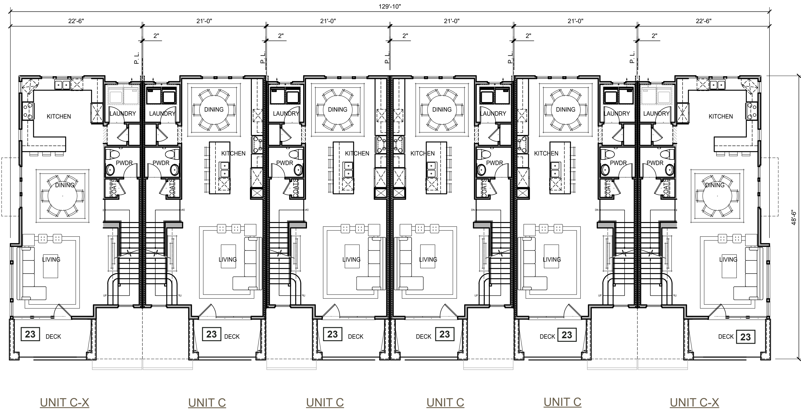
6-PLEX_3: SECOND FLOOR PLAN
